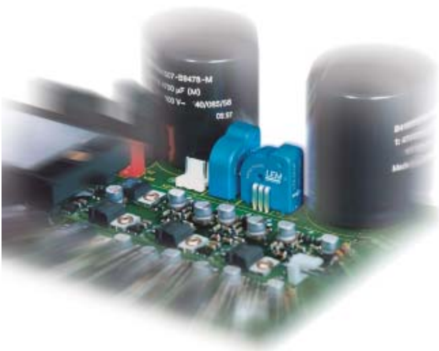
Figure 12 Use of the LTS series in an inverter for its regulation and protection. (Photo LEM, with the kind permission of REFU ELEKTRONIK GmbH)
