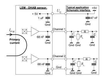
$R_{\rm L}$  > 10 kΩ optional resistor for signal line diagnostic  $C_{\rm L}$  < 100 nF EMC protection  $R_{\rm C}$  Low pass filter EMC protection (optional)
