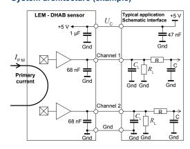
$R_{\rm L}$  > 10 kW optional resistor for signal line diagnostic  $C_{\rm L}$  < 100 nF EMC protection  $R_{\rm C}$  Low pass filter EMC protection (optional)
