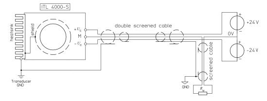
Figure 6: Double screened cable for long connection
