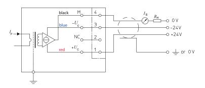
Figure 5: Connection principle
