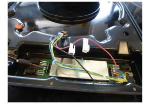
Figure 10: Remove the secondary winding short circuit
