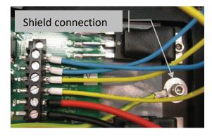
Figure 12: Connector X2 and shield connection
