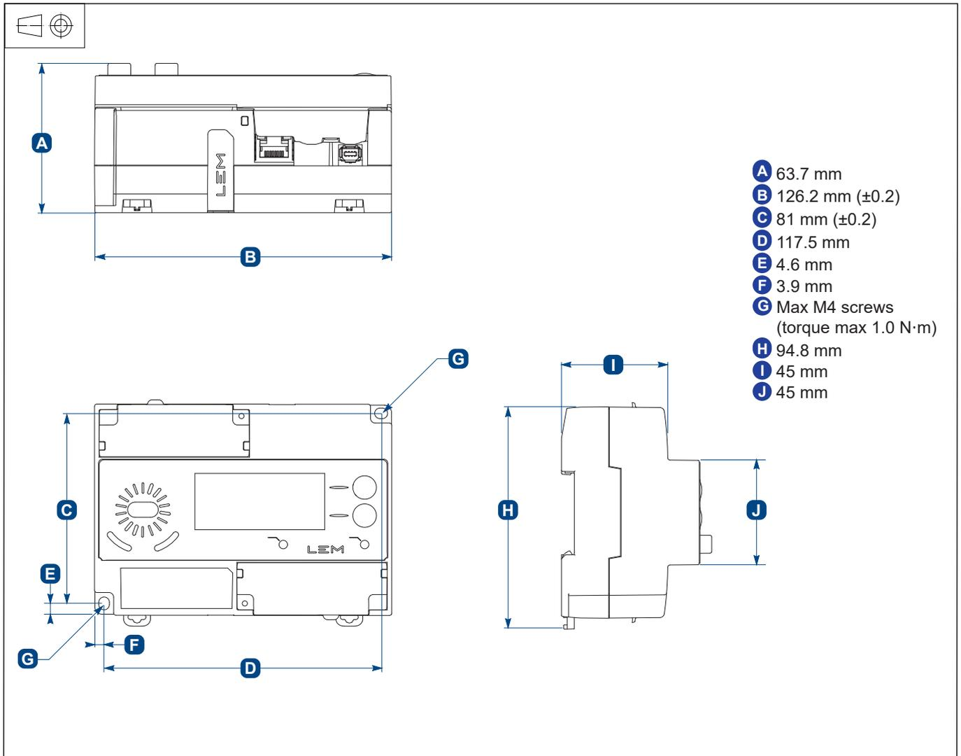
Sensor Unit dimensions (in mm)
