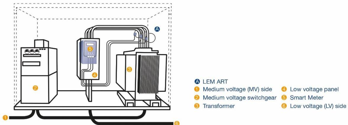
Within the MV/LV substation, the incoming power flow from the MV side (1) is managed by the MV switchgear (2) before being converted by the transformer (3) into LV (6). The smart meter (5) installed in the LV panel (4) measures the transformer’s (3) health with three independent current sensors – LEM ART (A). The ART allows safe commissioning of the smart meter on an existing live transformer.
