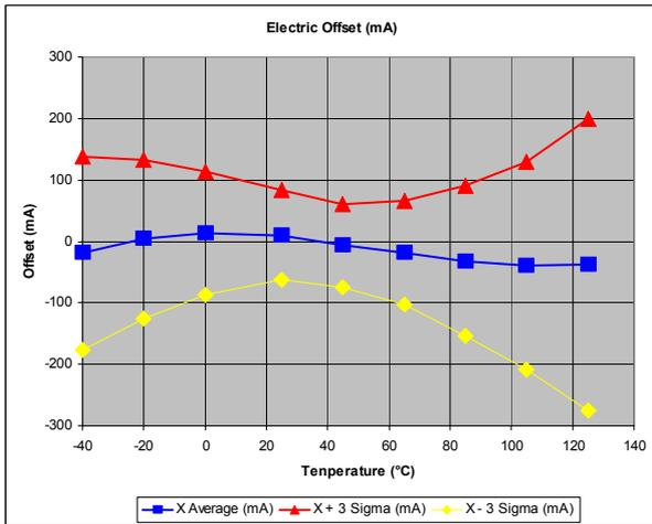
Figure 4-1 : Electric Offset Variation in Temperature
