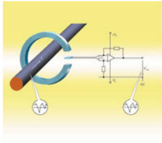
Figure 3-1: Open-Loop Hall-Effect Principle
