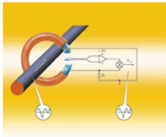
Figure 3-2: Closed-loop Hall Effect Principle
