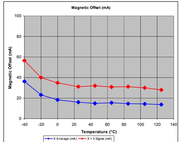
Figure 4-3 : Magnetic Offset Variation in Temperature
