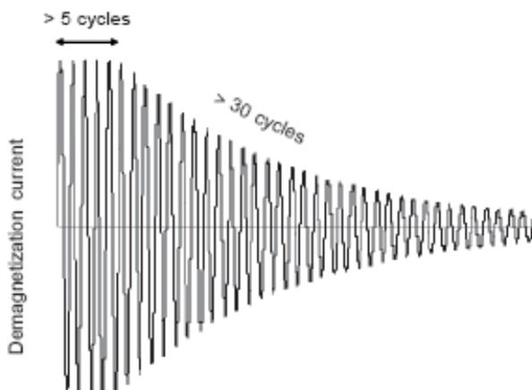
Figure 4-2: Degauss Cycle Current
