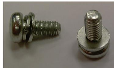
Moreover, the locking effect is based on the fact that tensile force, directly linked to the loosening torque, remains the same during time. This is true while tightening metal, but creeping is much more important for plastics. Therefore, even with the additional locking washer, loosening torque will decrease along time. We do not advise the use of locking washer as they are not very efficient for plastics (see Figure 11).
