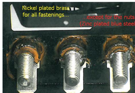
Fig. 14: Corrosion effect on transducer secondary connection with badly chosen nuts.
