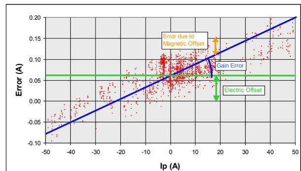
Figure 7-1: Transducer Output Error for Given Cycle
