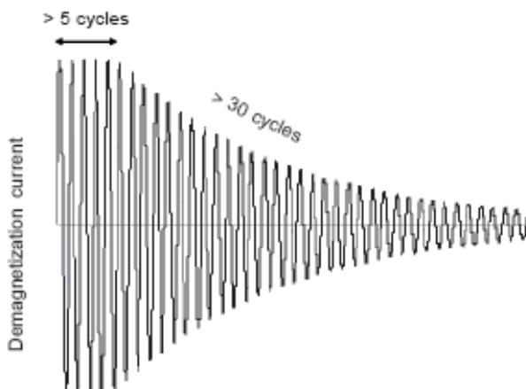
Figure 4-2: Degauss Cycle Current
