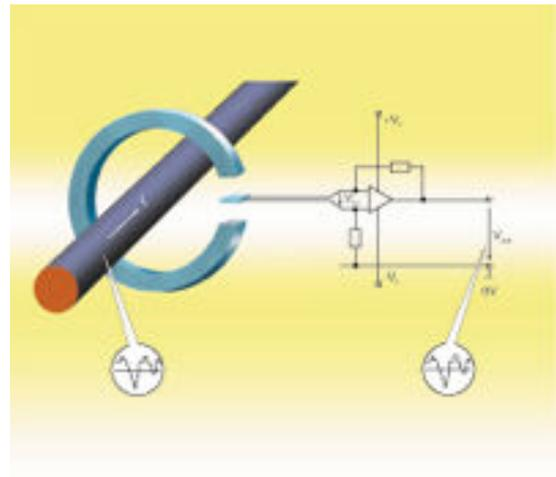
Figure 3-1: Open-Loop Hall-Effect Principle
