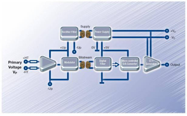
Fig. 3: DVM technology: Working principle of the insulating digital technology
