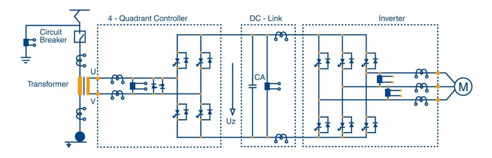
Fig. 1: The traction drive system
