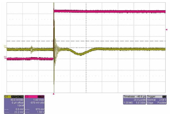
Fig. 5: DVM 4000 typical common mode behaviour against dv/dt of 6 kV/us (4200 V applied): Only 0.5% of  $V_{PN}$  as error generated with a recovery time of less than 50µs.
