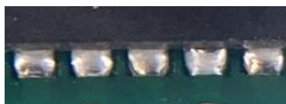
Figure 27: QFN with wettable flanks soldered on PCB
