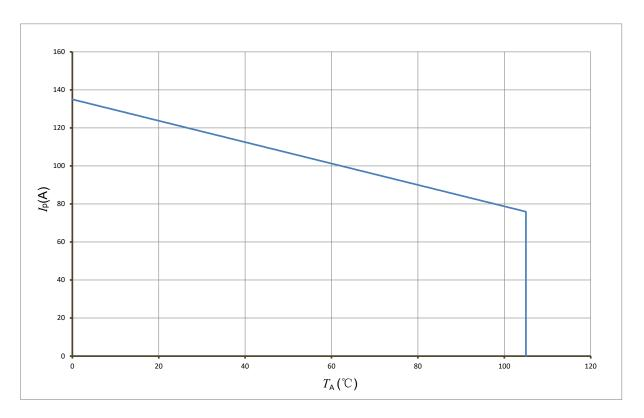
Figure 1:  $I_{\rm P}$  vs  $T_{\rm A}$  for CKSR 75-NP
