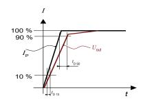
Figure 5:  $t_{\rm D\,10}$  (delay time @ 10 %) and  $t_{\rm D\,90}$  (delay time @ 90 %).
