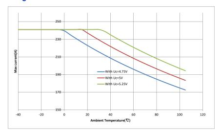
Figure 7: The measurement range vs. temperature
