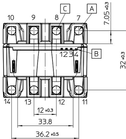
The four integrated primary conductors have a diameter of 4.5 mm.
