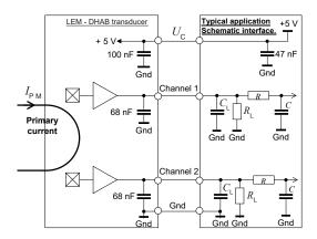
$R_{\rm L}$  > 10 k $\Omega$  optional resistor for signal line diagnostic  $C_{\rm L}$  < 100 nF EMC protection
