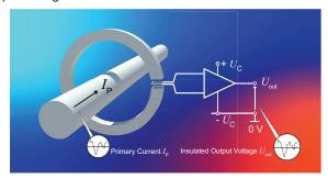
Fig. 1: Principle of the open loop transducer.
