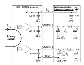
$R_{\rm L}$  > 10 k $\Omega$  optional resistor for signal line diagnostic  $C_{\rm L}$  < 100 nF EMC protection RC Low pass filter EMC protection (optional)
