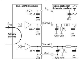
$R_{\rm L}$  > 10 k $\Omega$  optional resistor for signal line diagnostic  $C_{\rm L}$  < 100 nF EMC protection RC Low pass filter EMC protection (optional)
