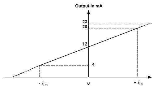
Note: <sup>1)</sup> The performance specified in the datasheet is valid within the 4-20 mA output range only.
