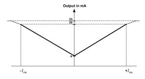
Note: 1) The performance specified in the datasheet is valid within the 4-20 mA output range only.
