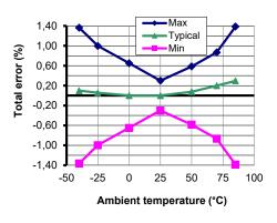
Figure 4: Total error in temperature
