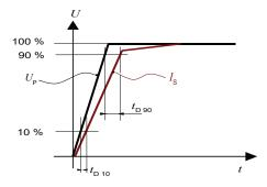
Figure 17: delay time  $t_{D 10}$  @ 10 % and delay time  $t_{D 90}$  @ 90 %.
