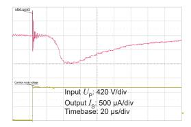
Figure 11: Typical common mode perturbation (1000 V step with 6 kV/µs  $R_{\rm M}$  = 100 Ω)
