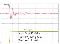
Figure 12: Detail of typical common mode perturbation (1000 V step with 6 kV/µs,  $R_{\rm M}$  = 100 Ω)
