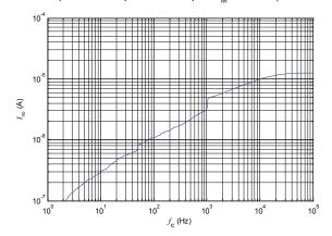
Figure 14: Typical total RMS noise current with  $R_{\rm M}$  = 50  $\Omega$ (fc is upper cut-off frequency of band low cut off frequency is 1 Hz)
