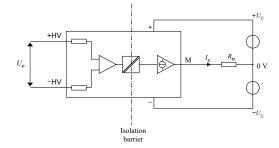
Figure 16: standard characterization schematics for current output transducers ( $R_{\rm M}$  = 50  $\Omega$  unless otherwise noted)
