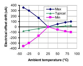
Figure 3: Electrical offset thermal drift
