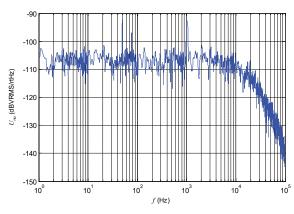
Figure 13: Typical RMS noise voltage referred to primary with  $R_{\rm M}$  = 50  $\Omega$
