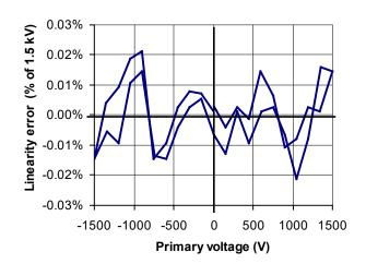
Figure 15: Typical linearity error
