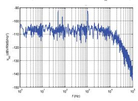
Figure 13: Typical output RMS noise voltage of U  $(R_{\rm M})$  with  $R_{\rm M}$  = 50  $\Omega$
