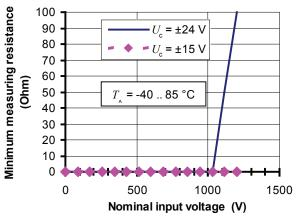
Figure 2: Minimum measuring resistance For  $T_{\rm A}$  under 80 °C, the minimum measuring resistance is 0  $\Omega$  whatever  $U_{\rm C}$
