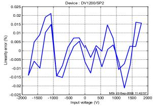
Figure 15: Typical linearity error
