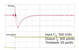
Figure 11: Typical common mode perturbation (1200 V step with 6 kV/ $\mu$ s  $R_{\rm M}$  = 100  $\Omega$ )
