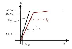
Figure 17: delay time  $t_{\rm D\,10}$  @ 10 % and delay time  $t_{\rm D\,90}$  @ 90 %.
