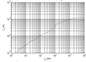
Figure 14: Typical total output RMS noise current with  $R_{\rm M}$  = 50  $\Omega$  (fc is upper cut-off frequency of band low cut off frequency is 1 Hz)
