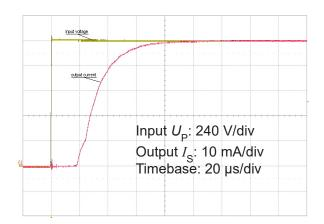
Figure 6: Typical step response (0 to 1200 V)
