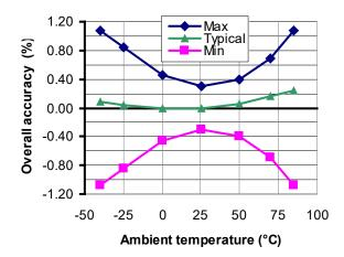
Figure 4: Total error in temperature
