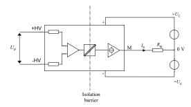
Figure 16: standard characterization schematics for current output transducers ( $R_{\rm M}$  = 50  $\Omega$  unless otherwise noted)
