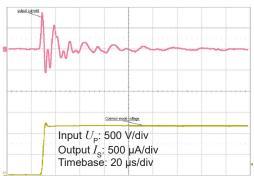
Figure 12: Detail of typical common mode perturbation (1200 V step with 6 kV/ $\mu$ s,  $R_{\rm M}$  = 100  $\Omega$ )
