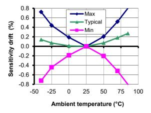
Figure 5: Sensitivity thermal drift
