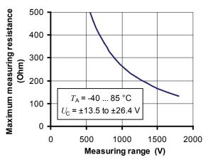
Figure 1: Maximum measuring resistance
