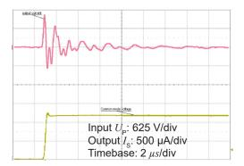
Figure 12: Detail of typical common mode perturbation (1500 V step with 6 kV/ $\mu$ s,  $R_{\rm M}$  = 100  $\Omega$ )
