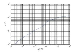
Figure 14: Typical total RMS noise current with  $R_{\rm M}$  = 50  $\Omega$ (fc is upper cut off frequency of bandpass, low cut off frequency is 1 Hz)
