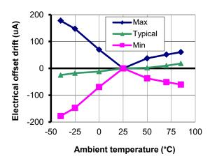
Figure 3: Electrical offset thermal drift
