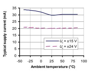
Figure 8: Supply current function of temperature
