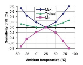
Figure 5: Sensitivity thermal drift
