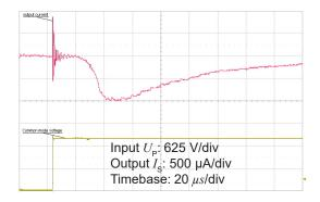
Figure 11: Typical common mode perturbation (1500 V step with 6 kV/ $\mu$ s  $R_{\rm M}$  = 100  $\Omega$ )
