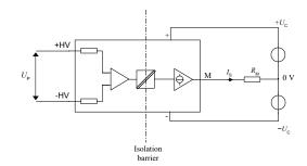
Figure 18: Standard characterization schematics for current output transducers ( $R_{\rm M} = 50 \ \Omega$  unless otherwise noted)
