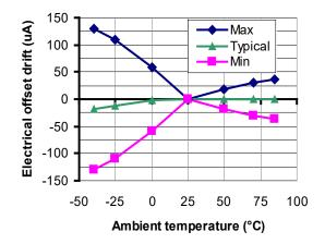
Figure 3: Electrical offset thermal drift
