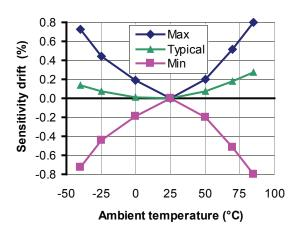
Figure 5: Sensitivity thermal drift
