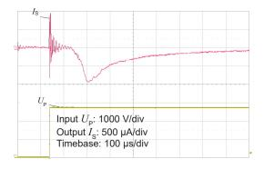
Figure 13: Typical common mode perturbation (2800 V step with 6 kV/ $\mu$ s  $R_{\rm M}$  = 100  $\Omega$ )
