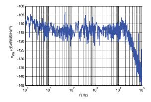
Figure 15: Typical noise voltage spectral density  $u_{no}$ referred to primary with  $R_{\rm M}$  = 50  $\Omega$
