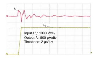
Figure 14: Detail of typical common mode perturbation (2800 V step with 6 kV/ $\mu$ s,  $R_{\rm M}$  = 100  $\Omega$ )
