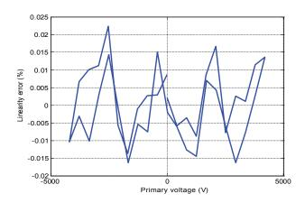
Figure 17: Typical linearity error
