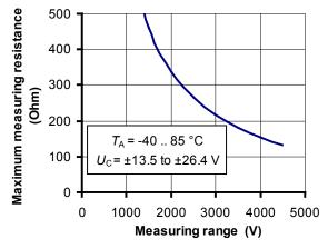
Figure 1: Maximum measuring resistance
