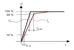
*Figure 19:* delay time  $t_{D10}$  @ 10 % and delay time  $t_{D90}$  @ 90 %
