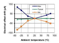
Figure 5: Electrical offset thermal drift
