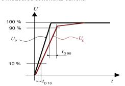
Figure 15: Delay time  $t_{\rm D\,10}$  @ 10 % and delay time  $t_{\rm D\,90}$ @ 90 %.
