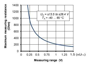
Figure 1: Maximum measuring resistance
