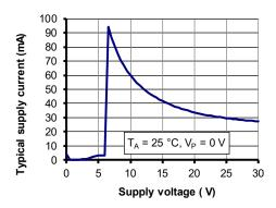
Figure 2: Supply current function of supply voltage
