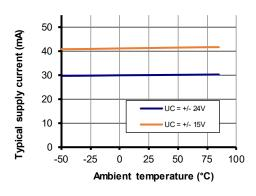
Figure 3: Supply current function of temperature
