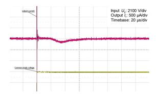
Figure 10: Typical step response (0 to  $U_{\mbox{\tiny PN}})$
