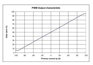
$$\begin{aligned} \textit{PWM period} \quad & T_{\textit{Period}} = T_{\textit{High}} + T_{\textit{Low}} \\ & \textit{PWM frequency} = \frac{1}{T_{\textit{Period}}} = 125\textit{Hz} \\ & \text{DutyCycle(\%)} = \frac{\mathsf{T}_{\textit{High}}}{\mathsf{T}_{\textit{Period}}} \times 100 \\ & \text{DutyCycle(\%)} = 50\% + \mathsf{G} \times \mathsf{I}_{\mathsf{P}} \text{ with G = Sensitivity (\%/A)} \end{aligned}$$
