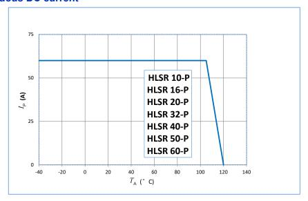
Important notice: whatever the usage and/or application, the transducer jumper temperature shall not go above the maximum ratings of 120 °C as stated in page 2 of this datasheet.
