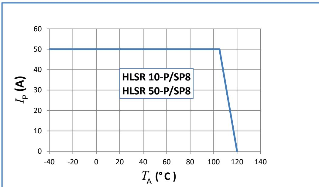
Important notice: whatever the usage and/or application, the transducer jumper temperature shall not go above the maximum ratings of 120 °C as stated in page 2 of this datasheet.
