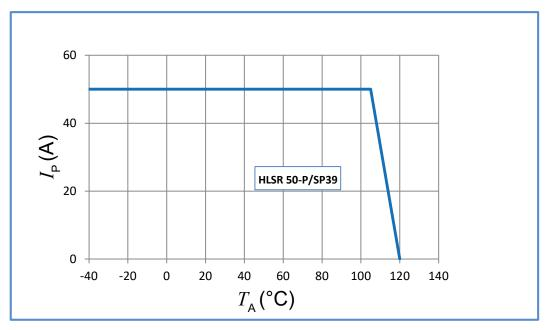
Important notice: whatever the usage and/or application, the transducer jumper temperature shall not go above the maximum ratings of 120 °C as stated in page 3 of this datasheet.
