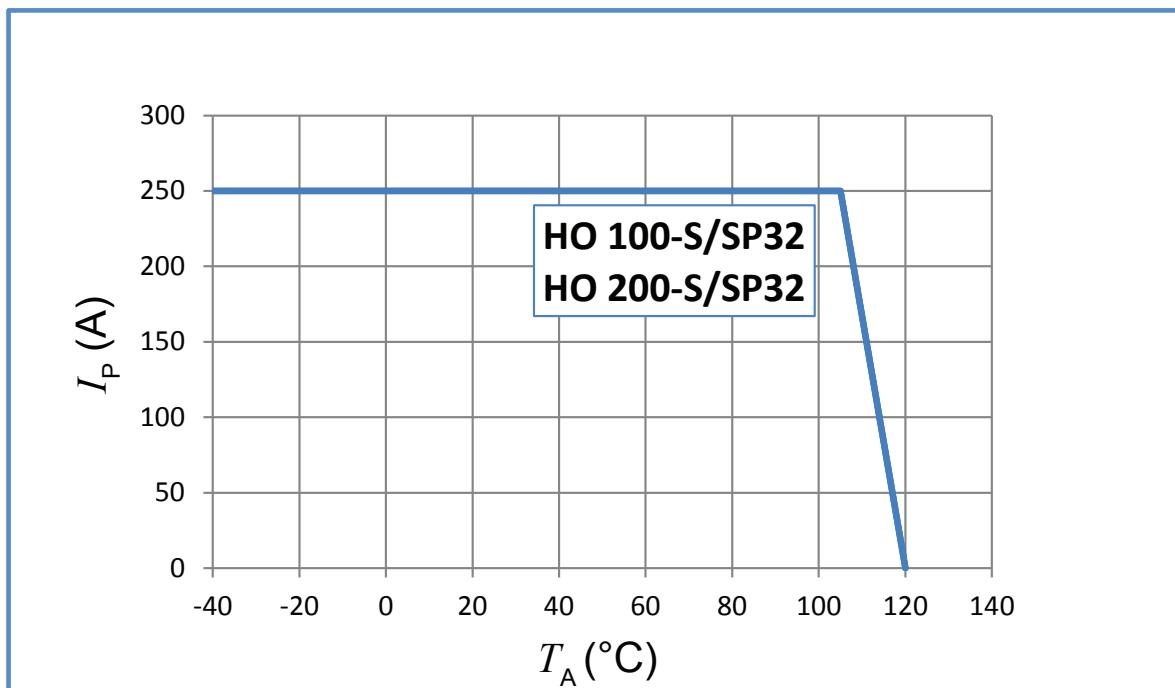
Important notice: whatever the usage and/or application, the transducer primary bar temperature shall not go above the maximum rating of 120  $^{\circ}\text{C}$  as stated in page 3 of this datasheet.
