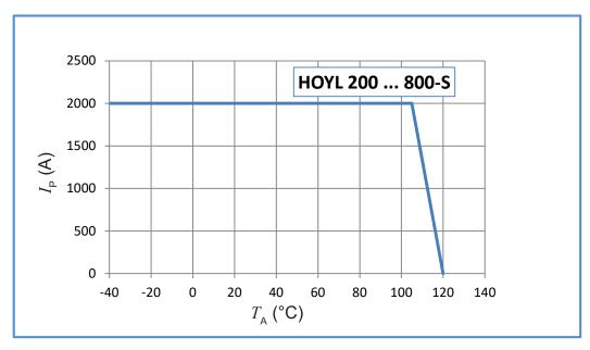
Important notice: whatever the usage and/or application, the transducer primary bar / jumper temperature shall not go above the maximum rating of 120 °C as stated in page 3 of this datasheet.
